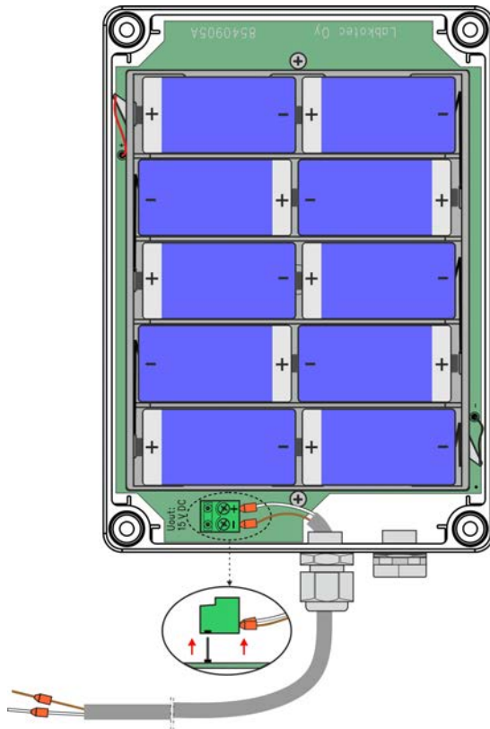
Figure 2 . Battery Box 10 installing batteries
